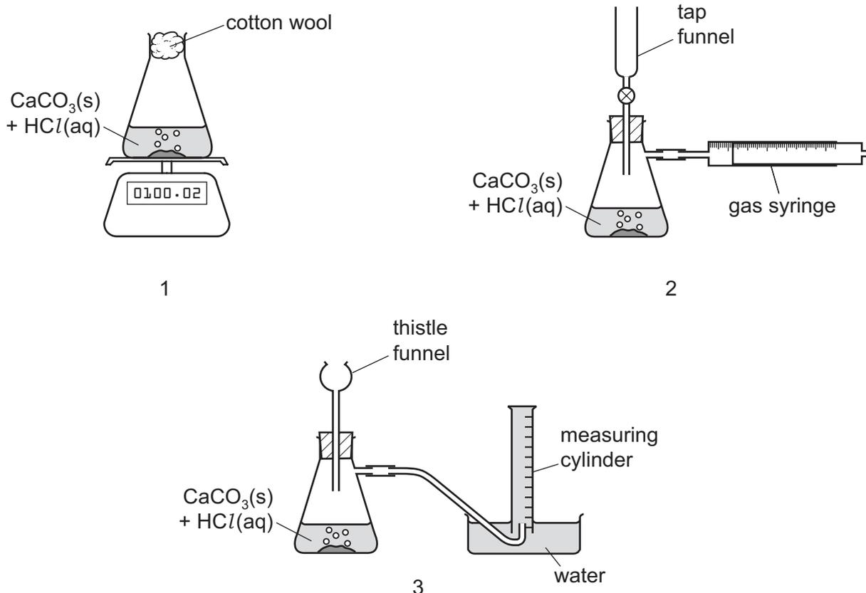
Which sets of apparatus are suitable, together with a stopwatch, for following the rate of this reaction?
